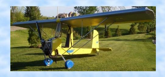
Wood with metal struts. Pilots legs extended outside the fuselage to the rudder pedals. Empty weight 250 lbs. Cruise 50 mph, stall 22 mph, and climb rate 700 fpm.
