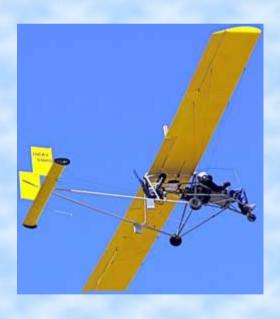
A Mark Stull design. Empty weight 245 lbs. Payload 255 lbs. 60 mph cruise with a stall speed of 28 mph and rate of climb 600 fpm.
