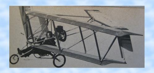
A 3-axis, open cockpit biplane. Empty weight 225 lbs. Payload 250 lbs. Stall speed 19 mph. 100 fpm climb rate. Load factors +6 Gs and -4 Gs.
