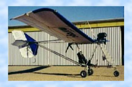
Designed by Frank Riley. Aluminum tube and sailcloth with tractor engine. Empty weight 246 lbs. Payload 254 lbs. Structural limits +5.6 Gs and -2.8 Gs.
