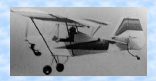
Designed by Fred Bell. Empty weight 252 lbs. Payload 346 lbs. Cruise speed 60 mph and stalls at 25 mph. Climb rate 800 fpm. Structural limits +6 Gs and -4 Gs.
