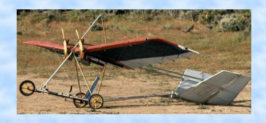
Designed by Ed Sweeney. Engines were Partner 8hp chain saws. Takeoff and landing speed was 15 mph and top speed was 55 mph. Empty weight 150 lbs.
