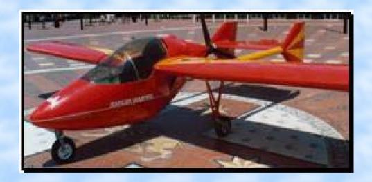
The first aircraft Mr. Sadler produced was all metal. Cruise speed 63 mph, stall speed 25 mph. Empty weight 245, payload 250 lbs, Structural limits +6 Gs and – 6 Gs.
