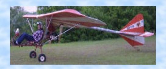
Homer Kolb designer. Single seat, twin tractor engines. Empty weight 185 lbs. Structural limits +4Gs and -2.5 Gs.
