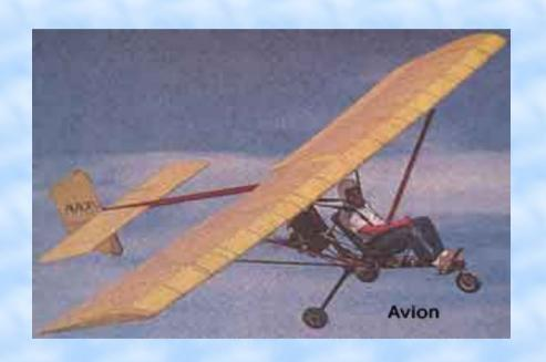
Designed by Bob Lovejoy. Cruise speed 48 mph, stall speed 27 mph. Load factors +6 Gs and-4 Gs. Empty weight 250 lbs. Payload 280 lbs.
