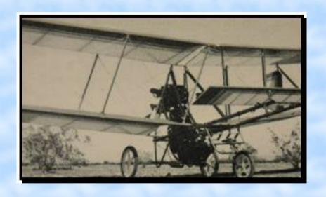
Designed by Kevin Bell. 38 hp engine. Cruise speed 45 mph and stall speed 23 mph. Climb rate 800 fpm. Requires 75-100 hrs. for construction. Empty weight 244 lbs. Useful load 225 lbs. Structural limits +5 Gs and -3 Gs.
