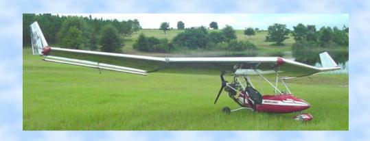
Designed by Don Mitchell. Powered glider from late 70's. Aluminum wing covering. Empty weight 280 lbs. Structural limits +4 Gs and -2.3 Gs.
