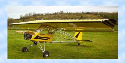
All welded aluminum construction. Wing swings parallel to fuselage for easy transport. Empty weight 254 lbs. Rate of climb 800 fpm.
