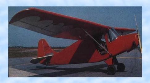
Designed by Mark Calder. Composite construction with Dacron covering. 28 hp 440A engine standard. Empty weight 241 lbs. Kit or plans built.
