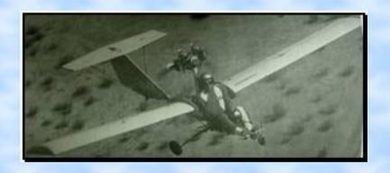
The PDQ-2 was designed by Wayne Ison. Empty weight 218 lbs. Cruise speed 70 mph and stall speed 46 mph. Rate of Climb 400 fpm. Rockwell JLO engine.
