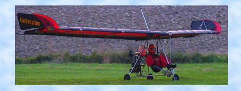
Designed by W. Kasper in collaboration with Steve Grossruck. Single-surface high-wing pusher engine monoplane with hybrid control. Empty weight 160 lbs. Structural strength +7 Gs and -4 Gs.
