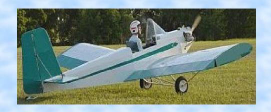
All aluminum aircraft that requires 600 hrs. build time. Structural loads are +4.4 Gs and -2.2 Gs. Empty weight 250 lbs.
