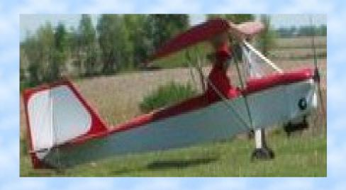
Designed by Scott Lane. Estimated build time is 300-500 hrs. 30 hp Kawasaki engine. Cruise speed 60 mph and stall speed 27 mph. Climb rate 650 fpm. Empty weight 249 lbs. Payload 250 lbs.
