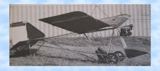
Developed by John W. Tucker. Cruise speed 40 mph, stall speed 20 mph. Climb rate 450 fpm. Empty weigh 250 lbs. Payload 275 lbs. Load factors +3 Gs and -3 Gs.
