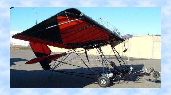
Designed by Dave Cronk. Empty weight 250 lbs. Load factors +5 Gs -3 Gs. Cruise speed 46 mph, stall speed 24 mph. Assembly time estimated at 30 to 40 hrs.
