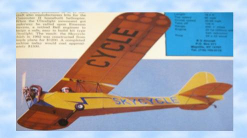
Single seat, parasol-wing monoplane. Empty weight 254 lbs. Payload 200 lbs. Load factors +3.5 Gs and -2 Gs. Cruise speed 40 mph, stall speed 27 mph. Climb rate 500 fpm.
