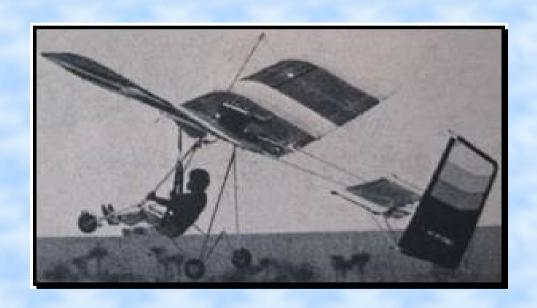
Aluminum tubing and sailcloth. Hybrid control system. Cruise speed 43 mph and stalls at 22 mph. Climb rate 800 ft/min. Empty weight 198 lbs.
