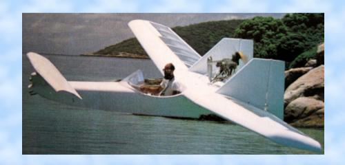
An amphibian in a pusher configuration. Canard with twin tail rudders. Retractable wheels. Empty Weight 240 lbs. Payload 230 lbs. Build time approximately 400 hrs.
