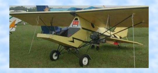
Designed by Jack Harper from materials purchased from the Home Depot. The plane utilizes all wood construction. Uses two 10 HP Tecumseh motors.
