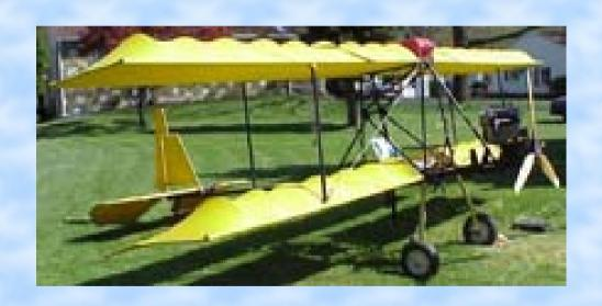
(Perfect Ultralight Plane). Designed by Lyle Matthews and sold as plans. Cruise speed 40 mph, stall speed 28 mph. Climb rate 600 fpm. Empty weight 248 lbs.
