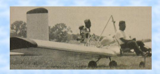
Designed by Richard Jiminez. Empty weight 234 lbs. Payload 271 lbs. Load factors +9 Gs and -4.5 Gs. Glide ratio 8:1
