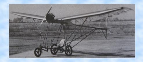
Designed by Jim Higgs. Empty weight 251 lbs. Structural limits +3.8 Gs and -1.5 Gs. Glide ratio 8:1.
