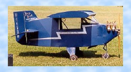
Designed by Donald Stits as World's Smallest Plane. Empty weight 250 lbs. Payload 188 lbs. Cruise speed 88 mph and climb rate of 925 fpm.
