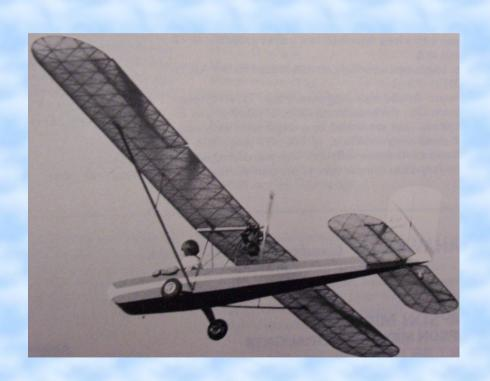
Designed by Bud Snyder. Essentially a motorized glider with a parasol wing. Empty weight 200 lbs, Payload 275 lbs. Glide ratio 15:1.
