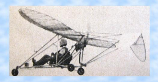
Designed by J. Bruce Emmons. Elliptical wing and inverted V-tail. Empty weight 165 lbs. Structural limits +9 Gs and -9 Gs. Glide ratio 15:1.
