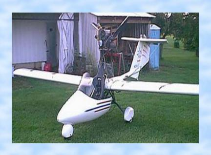
Designed by Gerald Nelson. Mid-wing monoplane of composite materials. Cruise speed 55 mph and stalls at 25 mph with a climb rate of about 500 fpm.
