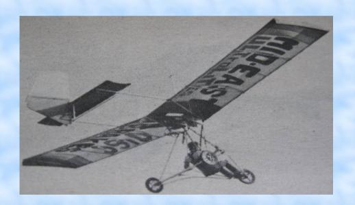
Weight shift control system. Single surface, wire braced wing. Empty weight 167 lbs.
