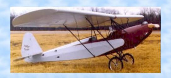
Constructed from gusset reinforced rectangular tubing. The fuselage weighs 12 lbs. Empty weight 250 lbs. Payload 270 lbs. Cruise speed 60 mph and stall speed 24 mph.
