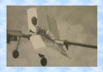
Pilot flies prone. Empty weight 175 lbs. Cruise speed 60 mph and stall speed 24 mph. Structural limits +6 Gs and -6 Gs. Glide ratio 14:1. 40 hr build time
