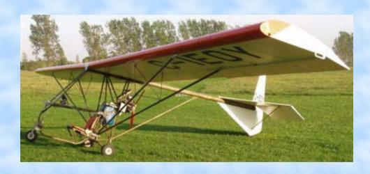
Single seat, pusher engine high wing monoplane. Aluminum tube and sailcloth covering. Empty weight 189 lbs. Build time 120-150 hrs.
