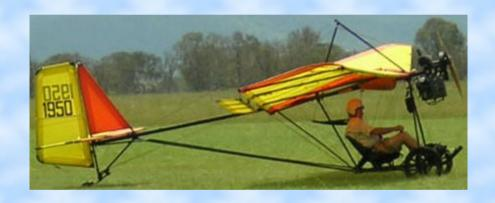
First major aircraft company to manufacture an ultralight airplane. Empty weight 220 lbs. Load factors +3 Gs and -2 Gs.
