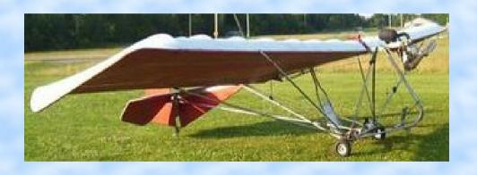
Plans built. Empty weight 160 lbs. Useful load 225 lbs. Building time 60-80 hrs. Cruise speed 38 mph and stall speed 20 mph. Climb rate 350 fpm.
