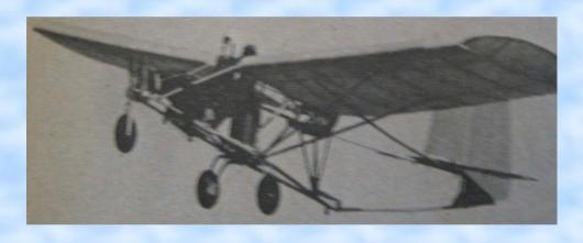
Designed by Larry Burke. Cruise speed 63 mph, stall speed 27 mph. Climb rate 750 fpm. Load factors +6 Gs and -3 Gs. Empty weight 250 lbs.
