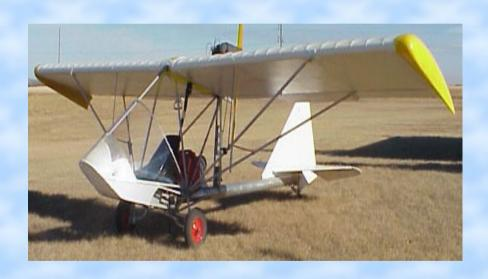
Single-seat, high-wing, monoplane. Empty weight 254 lbs. Build time 450 hrs. Plans only
