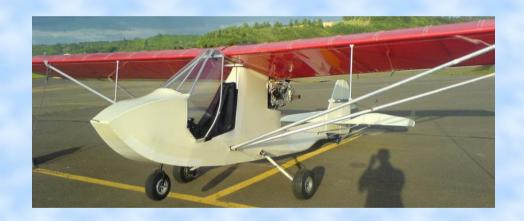
Factory built airframe and wings. Estimated 100 hours assembly time. Empty weight 235 lbs. Payload 258 lbs. Load factors +4 Gs and -3 Gs.
