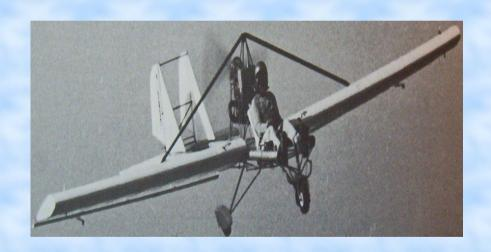
Designed by Jim Mead. Twin boom fuselages. Wood, tube and fabric construction. Structural limits +4 Gs and -4 Gs. Glide ratio 7:1. Empty weight 305 lbs
