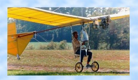
Designed by John Chotia and featured on Popular Mechanics cover in 1978. Empty weight 145 lbs. Maximum pilot weight 200 lbs. Stress limit +3.5 Gs. Construction time 250-300 hrs.
