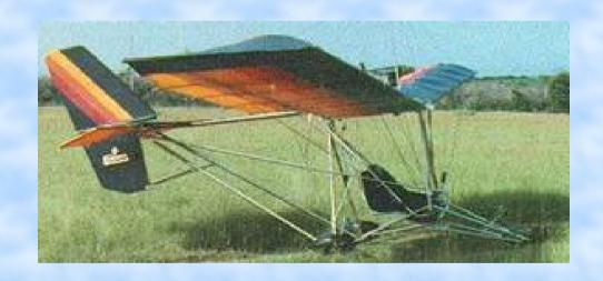
Designed by Wayne and Kerry Richter. Cruise speed 50 mph, stall speed 24 mph. and climb rate at 1000 fpm. Empty weight 235 lbs. Payload 280 lbs. Load factors +5 Gs and -3 Gs.
