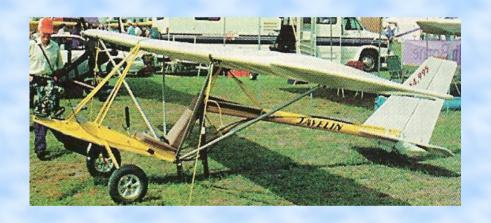
Cruise speed 60 mph, stall speed 26 mph. Climb rate 700 fpm. Estimated build time 80 hrs. Structural limits +4 Gs and -2 Gs. Empty weight 240 lbs.
