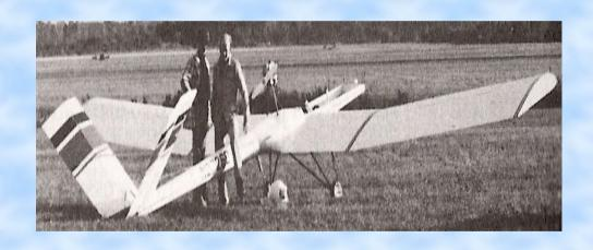
Designed by Emmett M. Talley. Aluminum and wood with 2-Axis controls. Empty weight 130 lbs. Glide ratio 15:1
