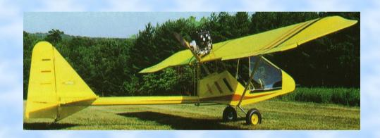
Designed by Homer Kolb. Empty weight 250 lbs. Payload 295 lbs. Structural limits +4 Gs and -2 Gs. Cruise speed 53 mph and climb rate 650 fpm.
