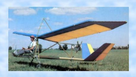
Klaus Hill designed monoplane with pusher engine and V-tail. 2-Axis control. Empty weight 185 lbs. Payload 255 lbs. Structural limits +4 Gs and -3 Gs.
