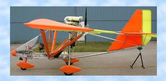
Assembled and ready to fly. Empty weight 250 lbs. Useful load 270 lbs. Cruise speed 55 mph and stall speed 28 mph. Structural limits are +4 Gs and -2.8 Gs.
