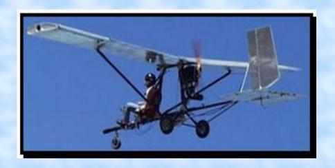
Bob Teman's design known for its toughness. Aluminum, steel and composite construction. Structural limits +10 Gs and -10 Gs. Empty weight 250 lbs. Payload 300 lbs.
