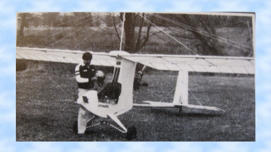
Single seat, pusher aircraft. Wood, tube and fabric construction. Empty weight 155 lbs. Payload 205 lbs. Structural limits +5 Gs and -3 Gs.
