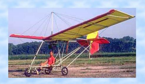
A Dick Turner design. Cruise speed 45 mph, stall speed 21 mph. Climb rate 800 fpm. Empty weight 200 lbs. Structural limits +5.8 Gs and -3 Gs.
