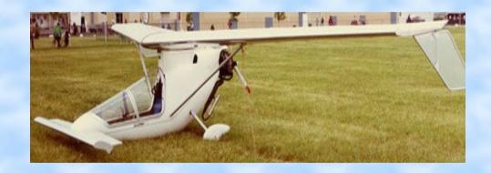
Designed by Romuald Drlik as a flying wing with canard. Empty weight 250 lbs. Payload 255 lbs. Load factors +5.8 Gs and -2.9 Gs.
