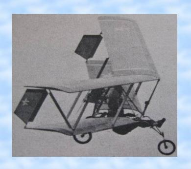
Originally flown by John Moody. Pusher bi-plane. Aluminum tube and sailcloth. Wire braced wing. Hybrid control system. Empty weight 120 lbs.
