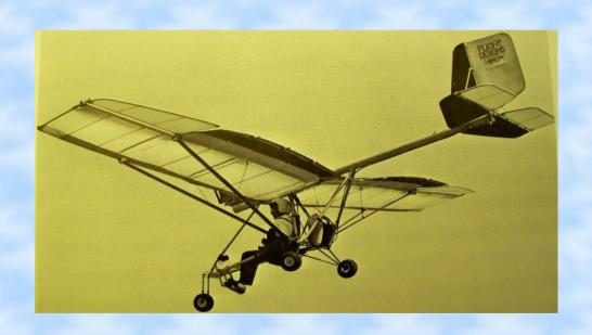
Cruise speed approx. 50 mph. Stalls at approx. 25 mph. Structural limits are +6 Gs and -4 Gs. Empty weight 247 lbs. Payload 253 lbs.
