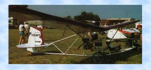
Designed by D. Paup. 2-axis control with pusher engine. Empty weight 165 lbs. Payload 237 lbs. Cruise speed 50 mph and stall speed 22 mph. Rate of climb 300 fpm.
