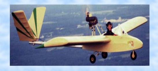
Designed by Nick Leighty and Rick Berstling. Single seat, mid-wing with V-tail. Empty weight 245 lbs. Payload 230 lbs. Structural limits +4 Gs and -4 Gs. Glide ratio 14:1.
