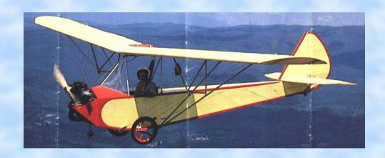
High wing parasol type aircraft with wood and fabric construction. Estimated 500 hr. build time. Empty weight 237 lbs. Cruise speed 50 mph and stalls at 27 mph. Climb rate 400 fpm.
