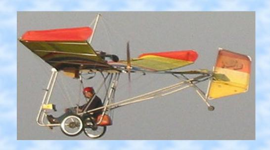
Designed by Bill Adaska. Empty weight 248 lbs. Structural limits +6 Gs and -3 Gs. 6. Glide ratio 8:1.
