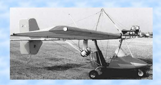
Designed by Donnie Eccker. Empty weight 249 Ibs. Payload 243 Ibs. Cruise speed 65 mph, stalls at 27 mph. Build time 100 hrs.
