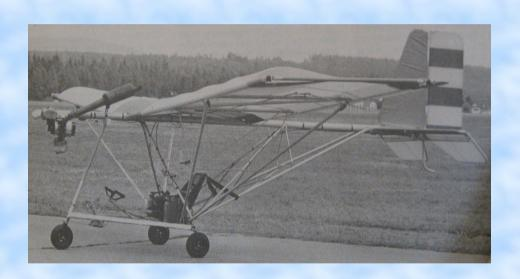
Tractor engine, aluminum tube monoplane with sailcloth wing. Empty weight 248 lbs. Payload 303 lbs. Structural limits +6 Gs and -4 Gs.
