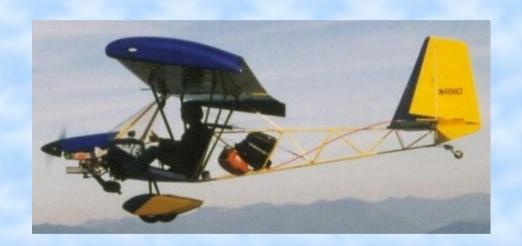
A conventional hi-wing monoplane and the pilot rides it like a bicycle. This is a 3-Axis aircraft with removable wings. Structural limits +4 Gs and -2 Gs.
