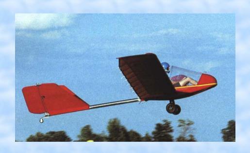
V-tail powered glider designed by Erwin Rodger and Delura Roger. Aluminum tube, and dacron sail cloth. Empty weight 252 lbs. Payload 252 lbs. Structural limits +4.2 Gs and -2 Gs.
