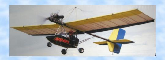
High-wing, 3-axis monoplane with cable braced wing. 30 hp Kawasaki 440 engine. Empty weight 252 lbs.
