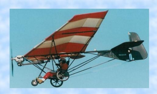
2-Axis control with tricycle landing gear. Empty weight 250 lbs. Payload 300 lbs. Cruise speed 55 mph and stall speed 20 mph. Rate of climb 1000 fpm.
