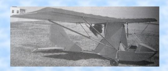
Designed by Clair O'Meyer. Empty weight 245 lbs. Payload 265 lbs. Load factors +4 Gs and -3 Gs. Cruise speed 48 mph and stall speed 20 mph.
