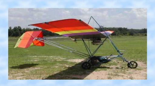
Designed by John Massey. 30 hp. engine. Breaks down to fit in a storage bag. Cruising speed 35 mph, stalling speed 25 mph, climb rate 800 fpm. Empty weight 253 lbs. Estimated 30 hr. construction time.
