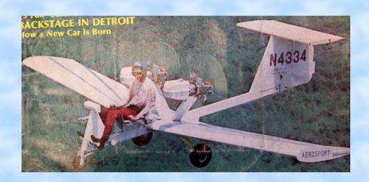
H.L. Wood is the designer. Easy build low wing monoplane. Rockwell JLO LB-600 snow mobile power plants weighing about 56 lbs and developing 33 hp.
