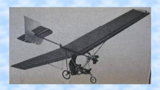
Powered glider with tractor engine.
