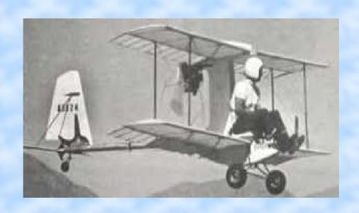
Designed by Bob Hovey. Essentially a plywood box filled with urethane foam. 14 hp McCulloch chainsaw engine. Cruise speed 40 mph, stall speed 26 mph, climb 100 fpm. Empty weight 123 lbs. Construction time around 400 hrs.
