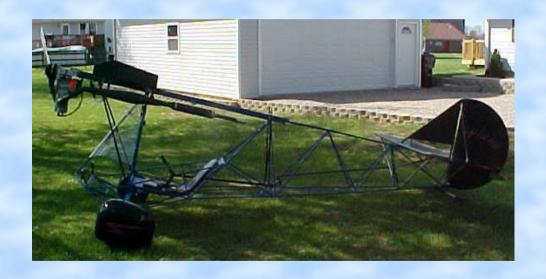
Designed by Ed Fisher. Triangular windshield. Fuselage comes already welded. Estimated 150 hrs. build time from kit and 600 hrs. from plans. Empty weight 225 lbs.
