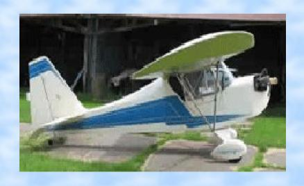
Single place, hi-wing monoplane. Empty weight 254 lbs. Payload 250 lbs. Cruise speed 58 mph and stall speed 26 mph. Climb rate 750 fpm.
