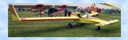
Designed by Craig Catto and Brian Glenn. Pusher engine with canard wing. Empty weight 220 lbs. Payload 260 lbs. Load factors +6 Gs and -4.5 Gs. Glide ratio 16:1.
